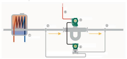
Fig. 42: Viscosity function returns a reference value used to activate a heating system (The above diagramm illustrates the fundamental functionality for one of several installation possibilities)
