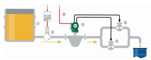
Fig. 41: Two-stage mode (The above diagram illustrates the fundamental functionality for one of several combination possibilities)
