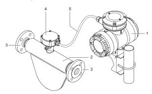
Fig. 6: Configuration of the Rotamass remote type
