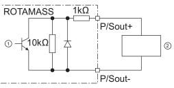
Fig. 36: Passive pulse or status output with switching amplifier connected in series
