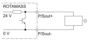
Fig. 33: Active status output P/Sout with internal pull-up resistor
