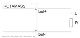
Fig. 26: Passive current output connection lout
