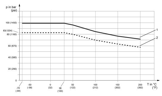
Fig. 14: Allowed process pressure as a function of process connection temperature
