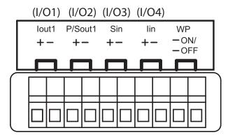
I/O1: lout1 Current output (active/passive)I/O2: P/Sout1 Pulse or status output (passive)
