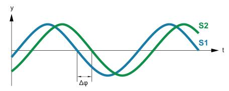
Fig. 3: Phase shift between output signals of S1 and S2 pick-offs
