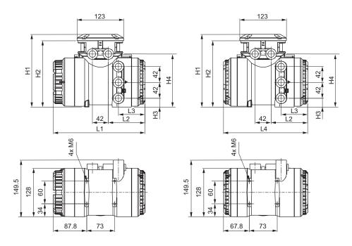
Fig. 22: Dimensions of transmitter in mm (left: transmitter with display, right: transmitter without display)
