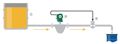
Fig. 40: One-stage mode (The above diagram illustrates the fundamental functionality for one of several combination possibilities)
