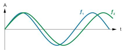
Fig. 4: Resonance frequency of measuring tubes
