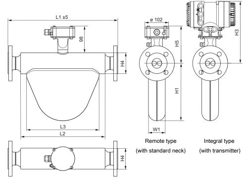
Fig. 21: Dimensions in mm
