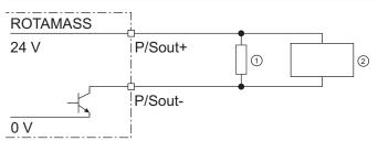
Fig. 27: Active pulse output connection P/Sout
