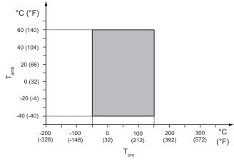
Fig. 18: Allowed process fluid and ambient temperatures, integral type
