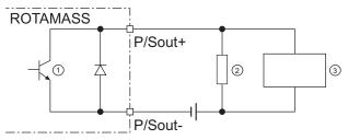
Fig. 30: Passive pulse output connection P/Sout with electronic counter
