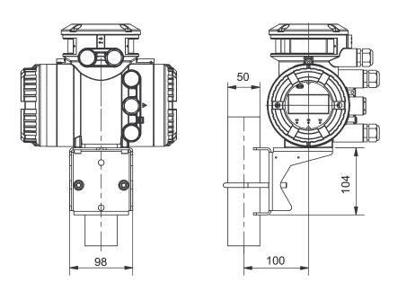
Fig. 23: Dimensions of transmitter in mm, attached by sheet metal console (bracket)
