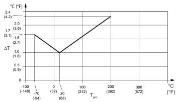
Fig. 10: Temperature accuracy
