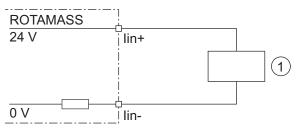
Fig. 37: Connection of external device with passive current output
