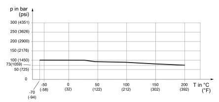
Fig. 17: Allowed process pressure as a function of process connection temperature
