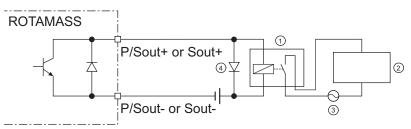
Fig. 35: Passive status output connection P/Sout or Sout for solenoid valve circuit
