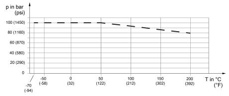
Fig. 15: Allowed process pressure as a function of process connection temperature, suitable for flange EN 1092-1 PN100
