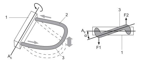
Fig. 2: Coriolis forces and measuring tube deformation
