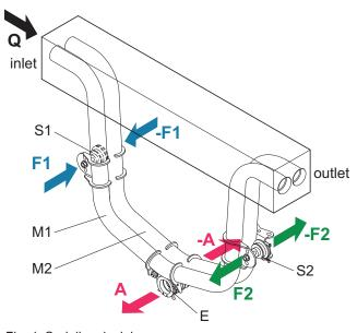
Fig. 1: Coriolis principle
