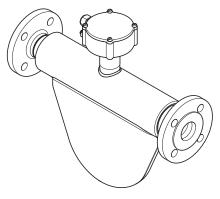
Fig. 20: Remote type sensor with standard neck
