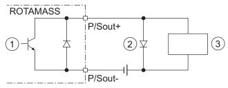
Fig. 31: Passive pulse output P/Sout connection with electromechanical counter
