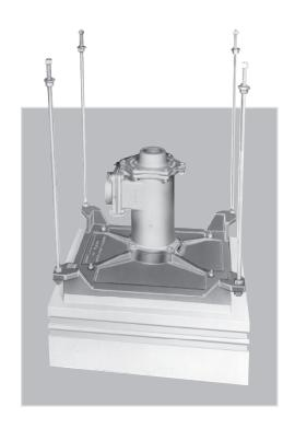
**Construction.** 4836 Burners have cast iron bodies and heat resistant iron mountings. All internals that see flame are stainless steel. Tiles are suitable for 3000 F tile temperature. Four hanger rods are furnished with each burner.
