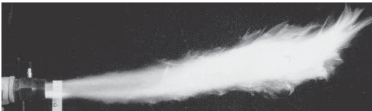
2½" 4020-HP Nozzle-Mix Pilot Tip 100% excess fuel 8 psi air pressure
