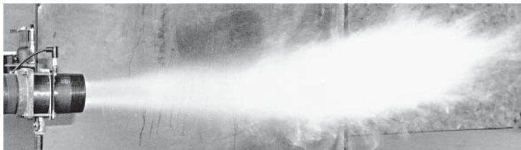
4" 4020-HP Nozzle-Mix Pilot Tip 100% excess fuel 8 psi air pressure
