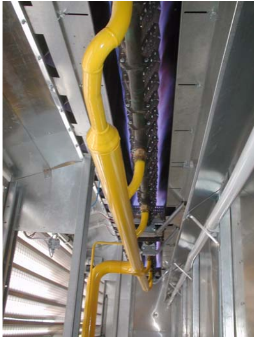
Direct air heating with NP-LE AIRFLO® burners in continuous flow dryers for grain
