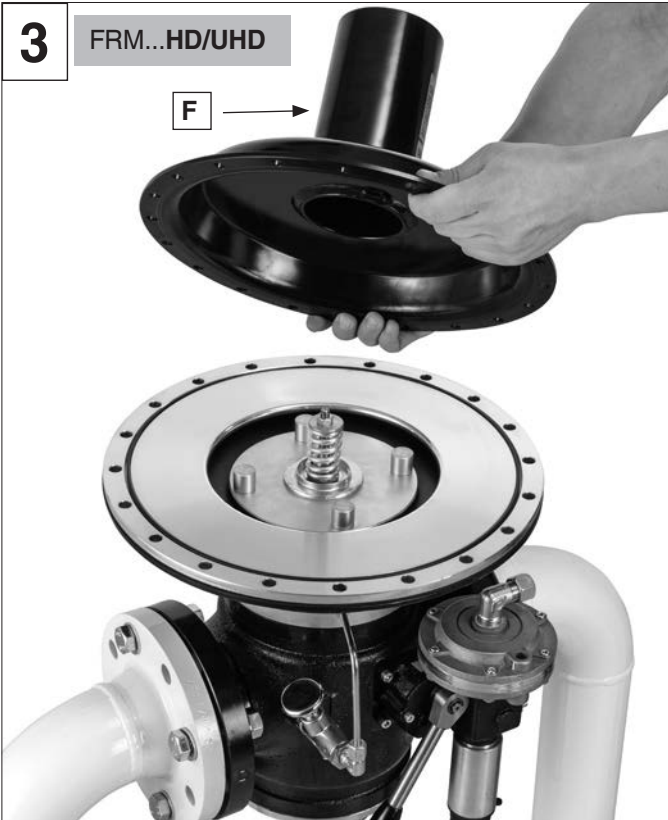
Remove the upper diaphragm shell F.
